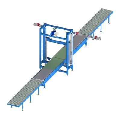
Standard configuration with moving belt (x axis) and up & down movable wire holding frame (y axis)
