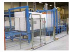
Models "more automated" which can be integrated inside the down-cutter of the automated cutting lines for sheets. These machines can be equipped even with systems for the automatic collection of the scraps on 4 sides (by suction devices) and further pre-crushing along the line, systems for automatic positioning of the cutting wires, etc...
